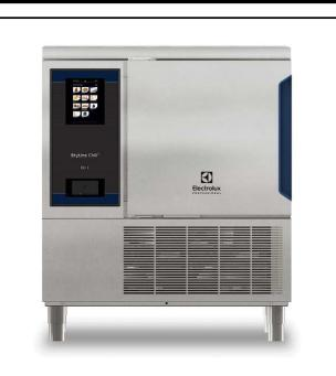
727905 (EBFA61THE) Skyline ChillS Blast Chiller Freezer 30/30kg, 6 GN 1/1 or 600x400mm (12 levels pitch 30mm) with touch screen control, Top and left hinged door
